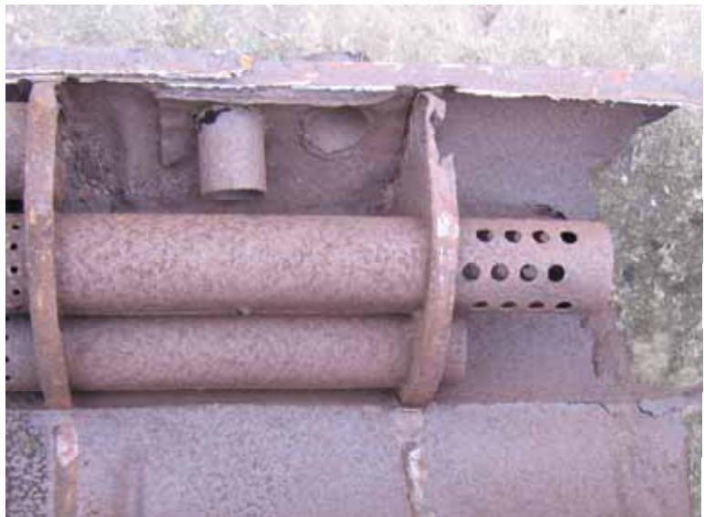
Here you see the outlet pipe, which is only 20 mm clear of the central resonator tube.
