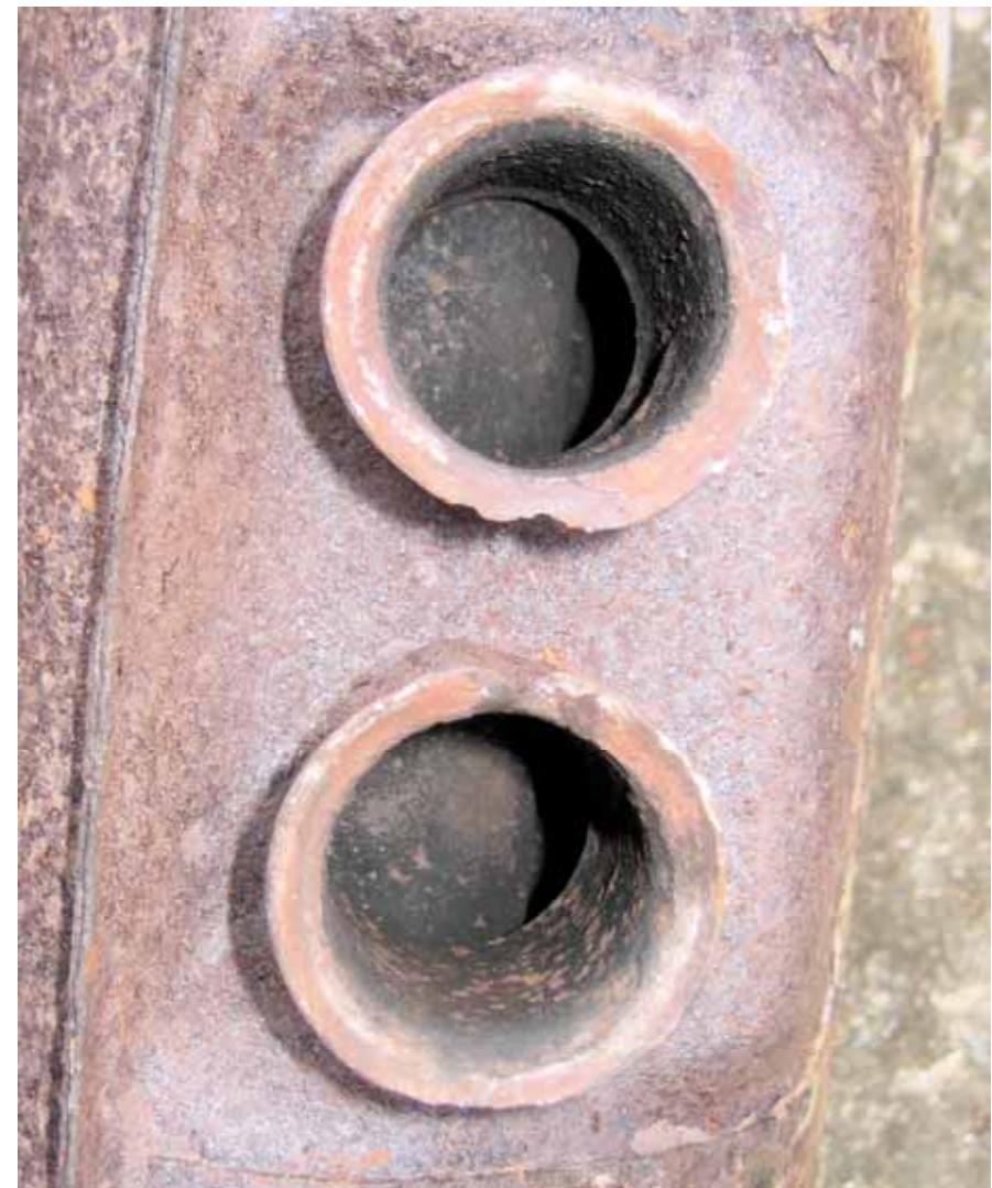
In the later silencer this weakness is a great deal worse: As you see the outlet pipes are also extended inwards, but now the inboard end lies much closer to the pipe inside. It is possible to reach with a finger only around half of the circumference of the outlet pipe.
